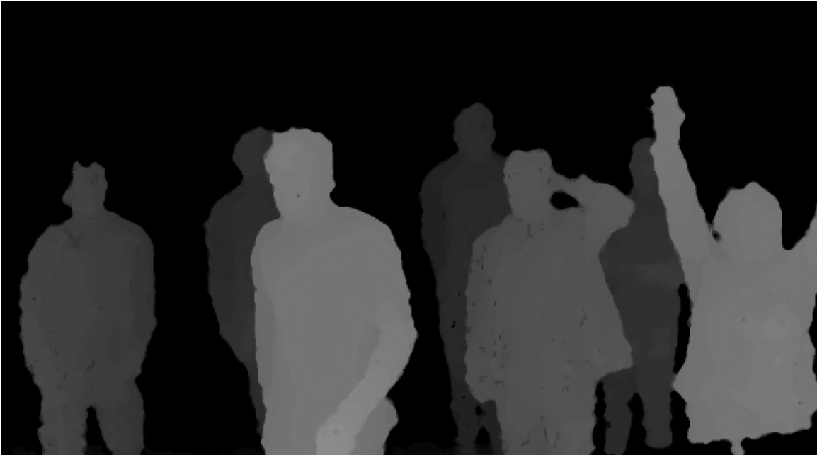
Figure 2.1: A depth image. The image intensity corresponds to how close the pixels are to the camera
