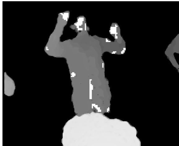
Figure 3.8: The body parts that are identified as hands by the algorithm. Many false positives are present
