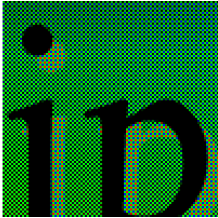
Figure 3: Example of a Bayer Image. (Colours are used to show the colour represented by each pixel) [wikipedia.org]
