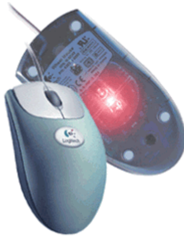
FIGURE 2: The Logitech iFeel mouse ( www.logitech.com ). The mouse looks and operates like an ordinary desktop mouse but contains a motor with an eccentric weight which generates a range of different types of simple vibrotactile feedback to the hand.
